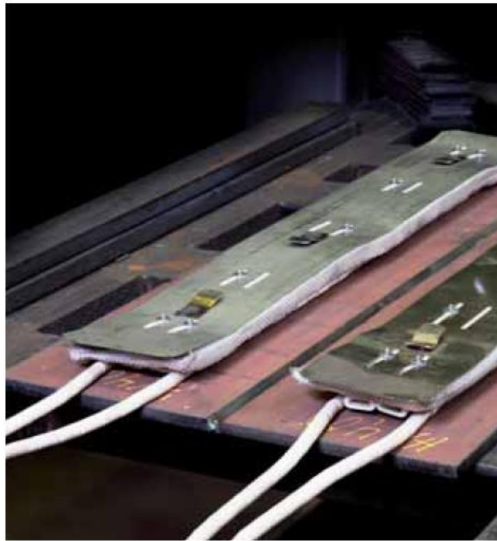
Using preheater elements
